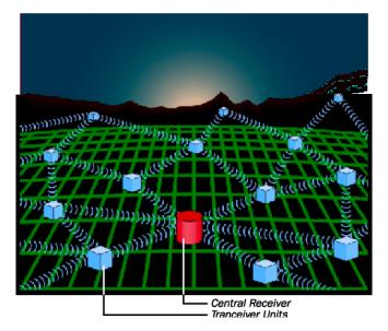
The Central Receiver is the primary receiving location of data for the network. The Central Receiver is a computer platform that integrates network management software and related applications to maximize network management. Each box indicates an SST in a remote location that sends and receives data from the Central Receiver and other SSTs to ensure a dynamic data path, which optimizes information flowing reliably across the network on a continual basis.
